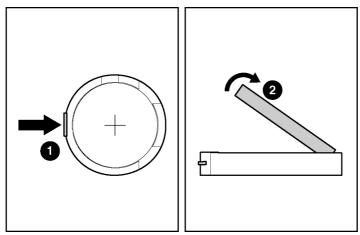
Figure G-2: Removing the existing battery
